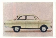
DKW 750 with two-cycle threecylinder engine, front-wheel drive, automatic clutch, about \$1,700
