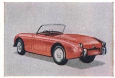
Austin-Healy Sprite sports car, 48-hp, 948-cc displacement, rack and pinion steering, \$1,795
