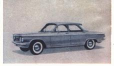
Corvair 700 four-door, 80-hp, air-cooled aluminum rear engine, 108-inch wheelbase, \$2,103
