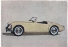
MGA 1600 roadster, 79.5-hp, rack and pinion steering, and Lockheed disc brakes, \$2,456
